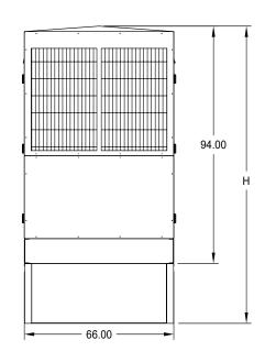
All enclosure models are 200 MPH wind rating certified in accordance with IBC2018 and ASCE/SEI 7-16 standards.
