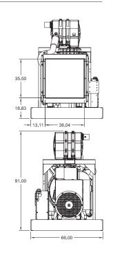
Drawings based on standard open power 480 volt standby generator. Lengths may vary with other voltages. Subject to change without notice. Sound data as measured at 23 feet (7 meters) in accordance with ISO 8528-10 at standby rating.
